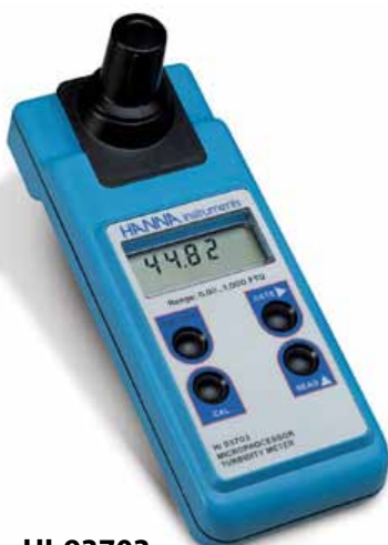
HI-93703 Turbidity meter 0.00 to 50.00 FTU or 50 to 1000 FTU
