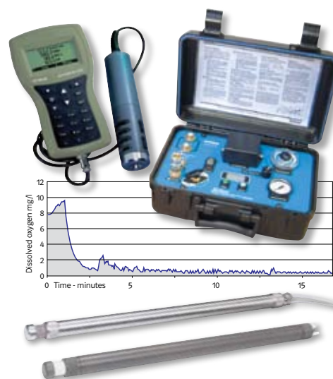
Above: Key equipment employed at Drigg. Solinst Integra™ Bladder Pumps and WQMP Multiparameter Water Quality Meter.
